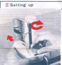
First, turn the Fastening Knob to left and let the Clamp down, and put the Wool Winder on the edge of the table as shown in the picture. Then fasten the Fastening Knob securely.
