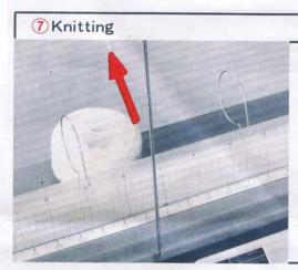
Place the wound wool under the Yarn Guide of the Tension unit and taking up the wool from outer side.
