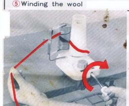
Holding the wool by left hand to give a small tension to it, turn the Handle to right so that you can wind up the wool into the ball.
