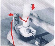
Thread the wool into the Yarn Guide and hook the end of yarn into the Gap of the Bobbin.
