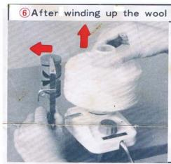
Open the Drum Arm to Left. And holding the top of the Bobbin, pull out the wound wool with Bobbin.
