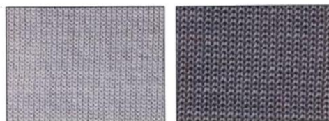
Lower tension knitting Higher tension knitting
