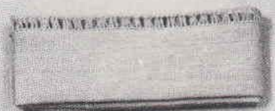
Cast-on Braid (two in number, one long and one short) For Automatic Casting-on.
