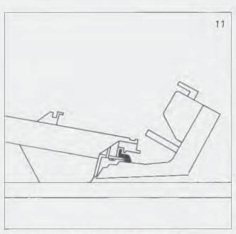
From the side insert the row counter into its support-rail exactly as shown in the illustration.
