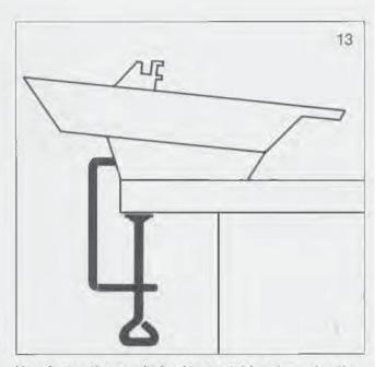
Now fasten the needle bed to the table edge using the two clamps.
