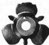
Wheel W 3 (3 large double teeth) every 3rd and 4th needle
