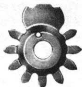
Wheel W 1 (1 large double tooth) every 11th and 12th needle
