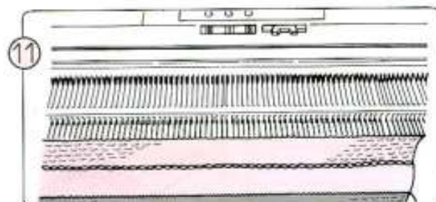
11 Set the Row Counter to 000 and knit the second half of the hem (i.e. the same number of rows as for the first half.)
