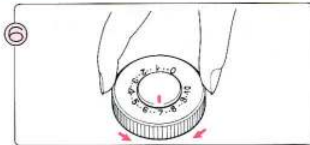
Set the Tension Dial using the Tension Chart on page as a guide.
