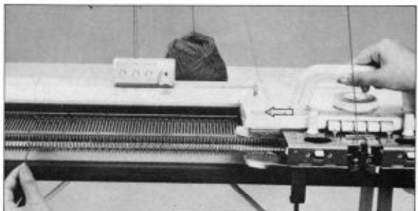
4. Thread the yarn into the yarn feeder "A". Holding the end of the yarn in your left hand, lay the yarn over the selected needles as shown. Hold the end of the yarn as shown in the figure.
