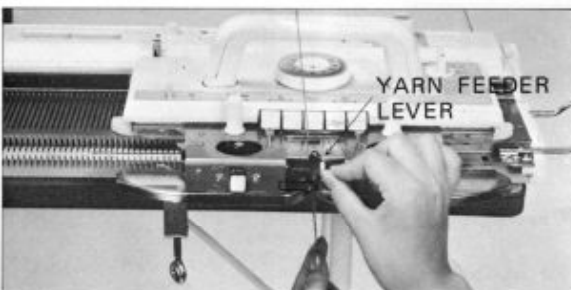
6. Hold the end of the yarn with your left hand under the YARN FEEDER "A". Close the YARN FEEDER LEVER.
