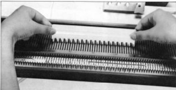
3. Using 1/1 NEEDLE PUSHER, bring forward every other needle to position D.
