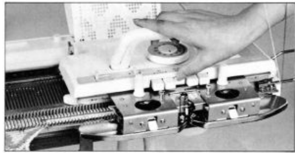
10. Push a cam button according to the pattern you are going to knit.
