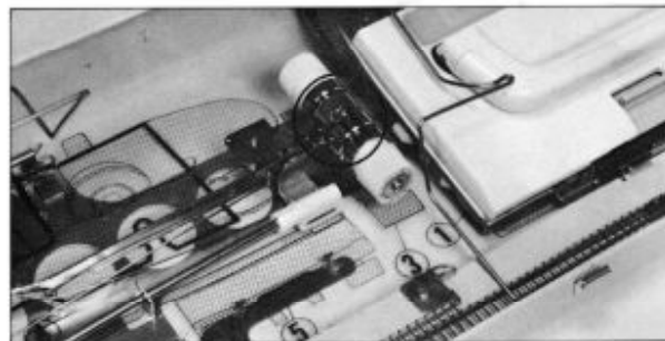
1). Set the A position of the YARN TENSION UNIT on the figure in carrying case.
