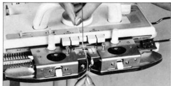
12. Thread the yarn into the YARN FEEDER and start knitting again. When knitting, Fair-isle patterns or Weaving patterns, do not forget to thread the second color yarn.
