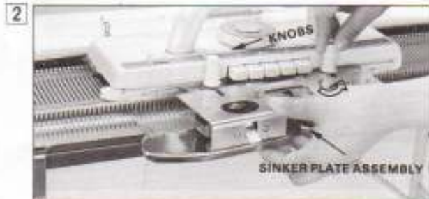
2 Loosen the KNOBS and remove the SINKER PLATE ASSEMBLY from the K CARRIAGE.
