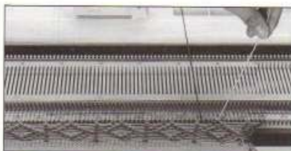
2-2) Pull the main yarn slightly sideways and up to unravel the knitting.
