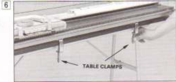
Fasten the machine to the table by tightening the TABLE CLAMP SCREW.
