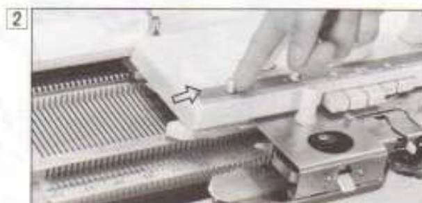
1 Knit one side in the same way as the plain knitting. Before you start knitting the first side, mark on the PUNCH CARD so that you can return to the exact row when you knit the other side.
