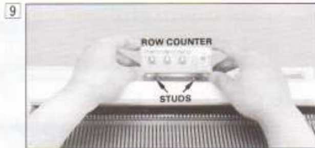
Set the ROW COUNTER up on the two STUDS at the center of the machine. 1) Set the ROW COUNTER onto the two STUDS.
