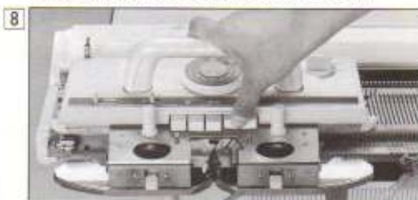
8 To select the needles, depress both "PART" buttons and set the CHANGE KNOB to K C.
