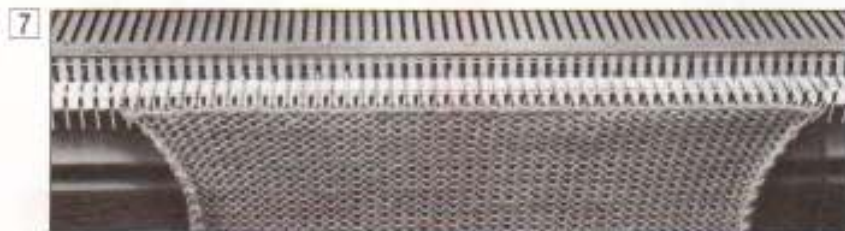
7 Now, the binding off is completed and piece can be removed from the machine.
