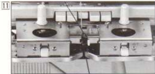
11 Thread the second color yarn which is clipped under the YARN CLIP into YARN FEEDER "B" without opening the YARN FEEDER LEVER. Hold the Yarn under the YARN FEEDER with your left hand.
