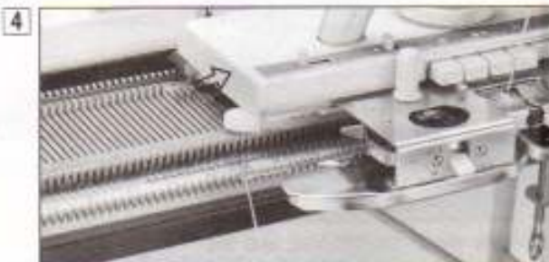
4 Pull down the fabric by left hand, and move the carriage by right hand.
