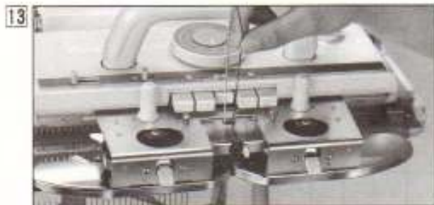
13 Thread the yarn into the YARN FEEDER and start knitting again. When knitting, Fair-isle patterns or Weaving patterns, do not forget to thread the second color yarn.
