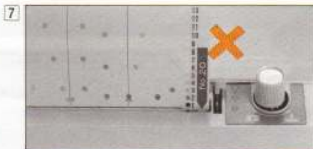
7 When knitting Lace patterns or Fine-Lace patterns do not set the CARD LOCK LEVER to the "▽" mark.
