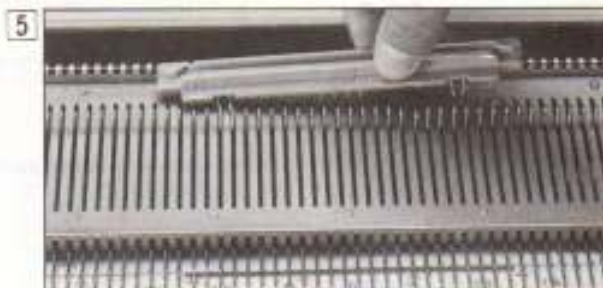
5 Place the ONE-POINT CAM at the needle bed by adjusting to the ▶ marks on the Rear rail and ONE-POINT CAM.
