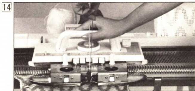
14 Operate the K CARRIAGE pulling the yarn slightly up.
