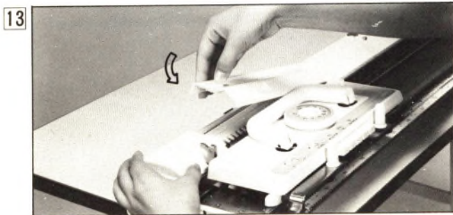
Replace the other accessories in the accessory box and close it. Push all needles back to position A.
