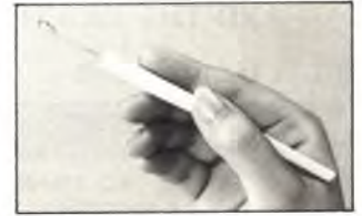
How to hold the latch tool.
