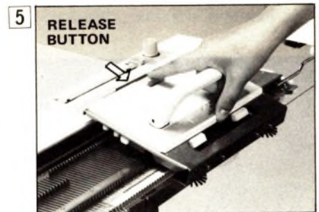
5 Remove the L CARRIAGE from the machine by pushing the RELEASE BUTTON.
