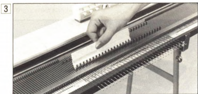
3 Using 1/1 NEEDLE PUSHER, bring forward every other needle to position E.
