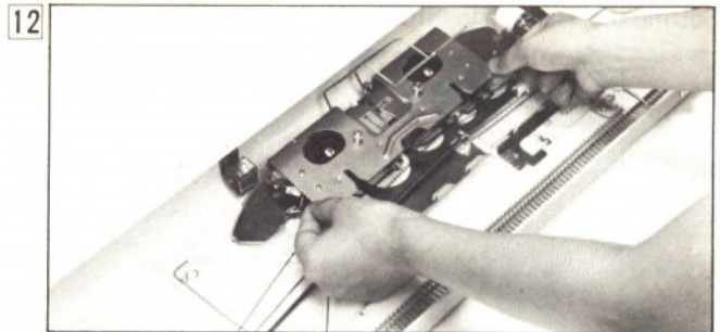
Remove the SINKER PLATE ASSEMBLY from the carrying case.
