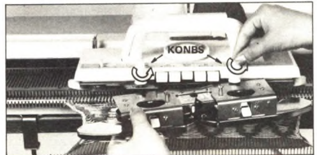
2) Loosen the KNOBS and remove the SINKER PLATE ASSEMBLY from the K CARRIAGE.
