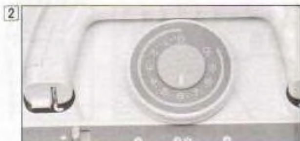
2 It is recommended to use one number lower than original tension.
