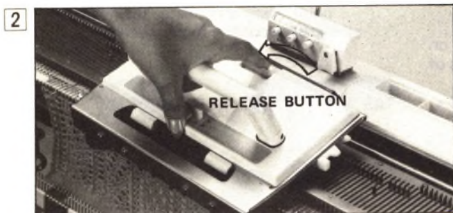
Push the RELEASE BUTTON toward you to remove the L CARRIAGE. If the L CARRIAGE is caught on the needles, take care in removing it.
