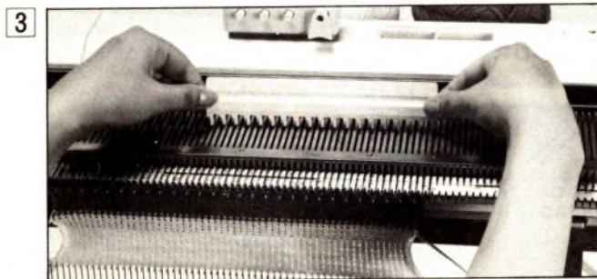
3 Starting with the second needle from either end, bring forward every alternate needle to position D by using the 1/1 NEEDLE PUSHER. End needles must remain in position B.
