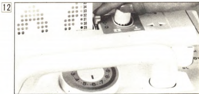
12 Set the CARD LOCK LEVER to the "▼" mark.
