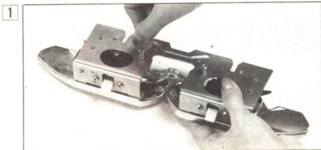
1 Change the yarn feeder to the PLATING YARN FEEDER. (See page 62)
