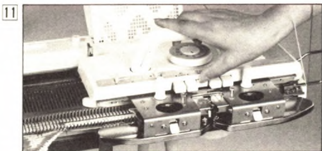
11 Push a cam button according to the pattern you are going to knit.
