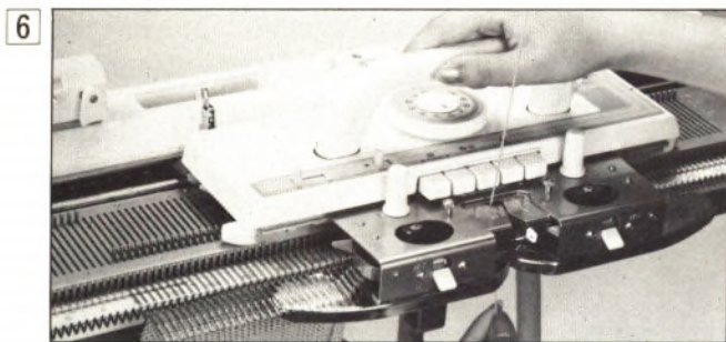
6 Thread the yarn into YARN FEEDER A and knit the other side of the neck and shoulder for part ③
