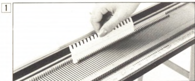
1 Bring forward the required needles to position B.
