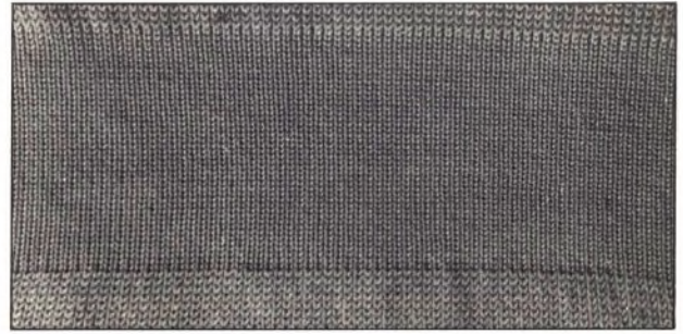
2) TENSION DIAL is loose.
