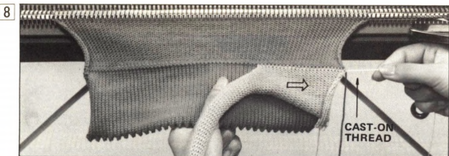
8 After knitting several rows, pull out the CAST-ON THREAD. The part knitted with waste yarn is removed. Then you have made a PICOT HEM.
