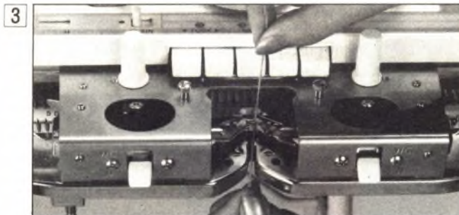
3 Thread the main yarn into the main yarn feeder. Knit several rows of plain knitting and place the K CARRIAGE on the right side of the machine.
