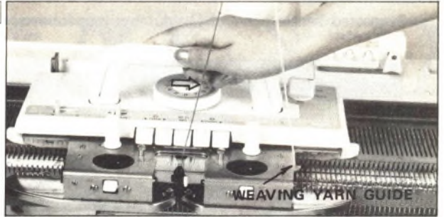
Move the K CARRIAGE to right making sure that the Weaving yarn is in the right WEAVING YARN GUIDE.
