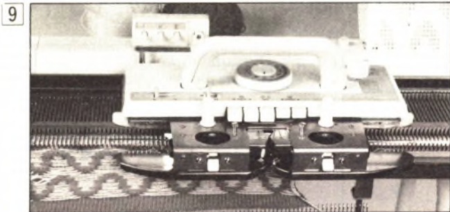
9 Operate the K CARRIAGE. At this time, the yarn is not in the yarn feeder.
