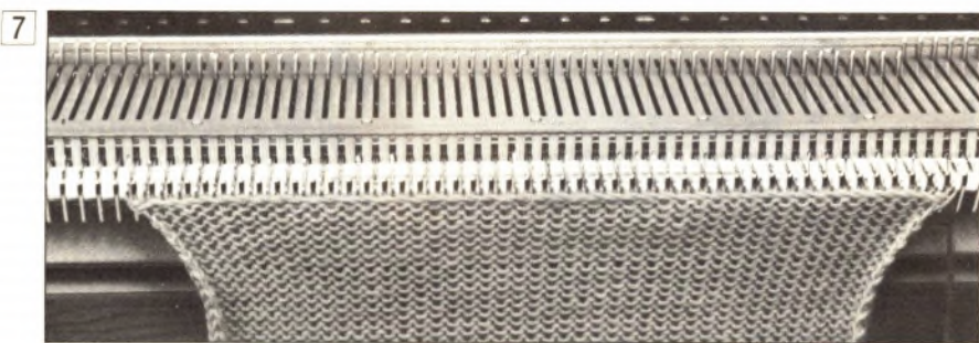
7 Now, the binding off is completed and piece can be removed from the machine.
