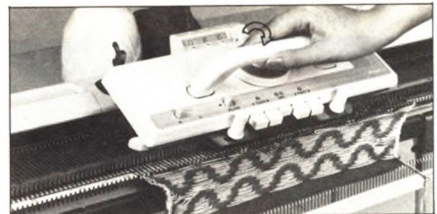
Lift up the K CARRIAGE to remove.
