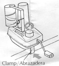
Turn the Drum Holder to the arrowed direction as far as it will go.
