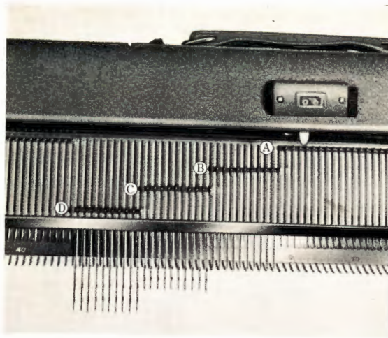
The Relation Between the Needle Positions, Cams and Russel Buttons
