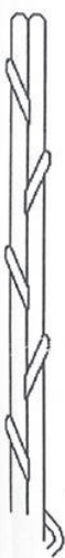
DIAGRAM 2 - JOINING RIBS Seam closed by gently pulling together as sewing is being done.
