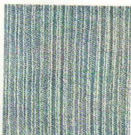
2X1 RIB KNITTING 2 RECHTS-1 LINKS TRICOTAGE DE CÔTES 2X1
