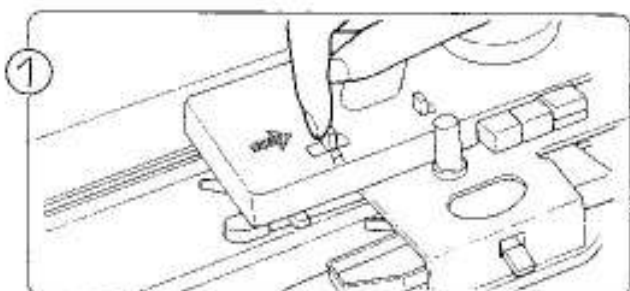
Set the Holding Cam Lever to H and the Cam Buttons and Change Knob according to the pattern.
