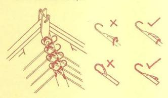
Lay yarn across "V" formed by the needles and through yarn guides at opposite end. Unwind yarn from the ball or cone.
