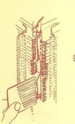
Push stitches clear of needles and floats down centre using stitch size guide.
