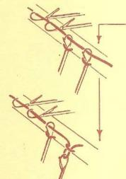
Knit, partially lowering pairs of needles until latches close, then lowering each in turn completely.
