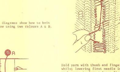
Hold yarn with thumb and finger whilst lowering first needle in each group to form a loose float. This enables knitting to expand when removed from the frame.
