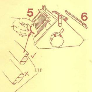
ALWAYS ASSEMBLE WITH THE LIP FACING UP THE FRAME UNTIL YOU HAVE TRIED THE STITCH SIZE PRODUCED AND NEED TO TURN THE BAR ROUND TO GET SMALLER STITCHES
