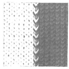
The link between each different colour is obtained by crossing both yarns between two needles.
