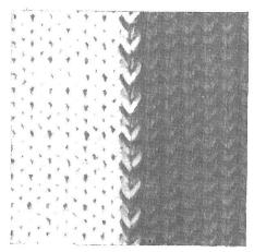
The join between each different coloured yarn is obtained by knitting both yarns on the same or common needle.
