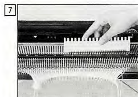
After picking up all the stitches, bring the needles to position E. Knit one row.
