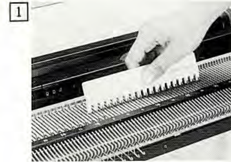
1 Using the 1/1 NEEDLE PUSHER bring forward to position E the required number of needles, after selecting an equal number of needles on either side of the center "0". Refer to the way how to cast-on and start knitting on p.p. 9 ~ 11.
