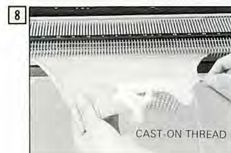
Pick up the stitches in the same way as for the plain hem and hook them onto the empty needles.
