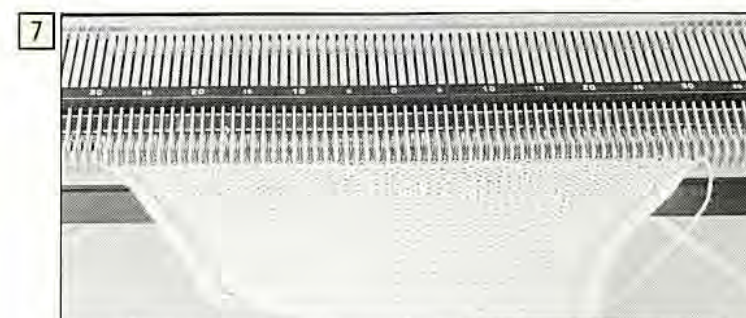
Now, the binding off is completed and the knitting switch can be removed from the machine.
