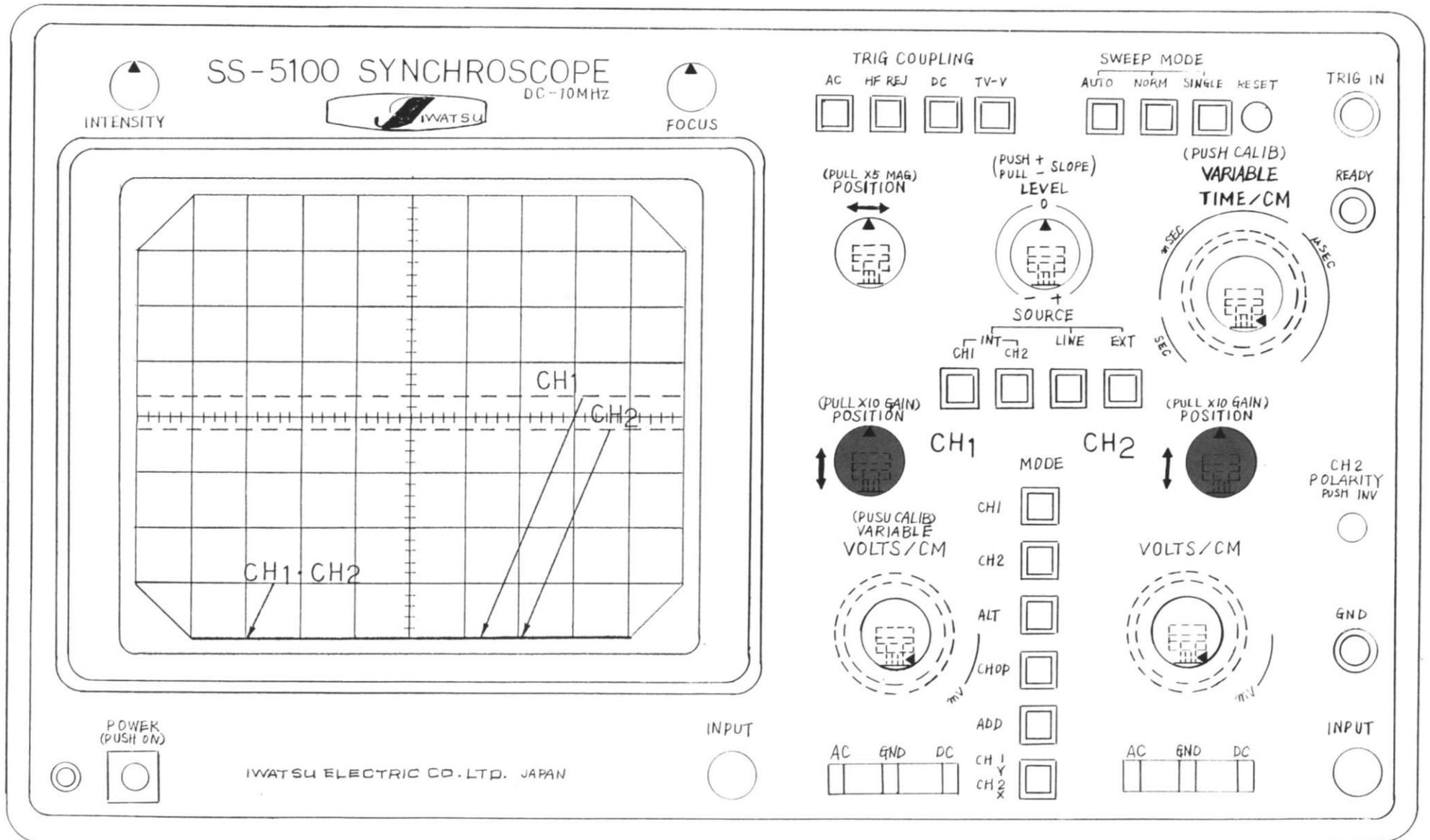
2. SETTINGS FOR CHECKING THE PCP SIGNAL
