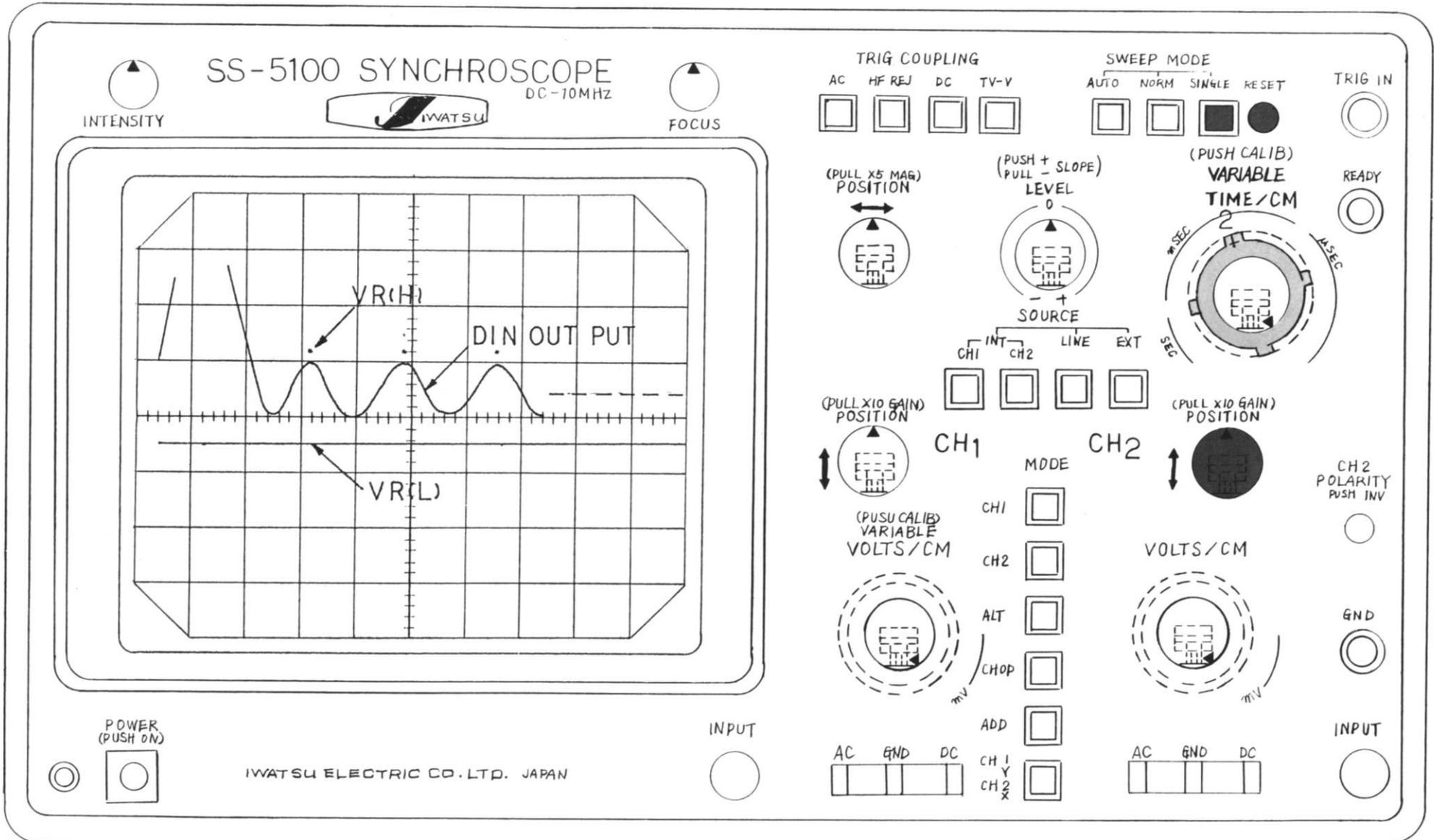
4. SETTINGS FOR CHECKING THE PSD SIGNAL
