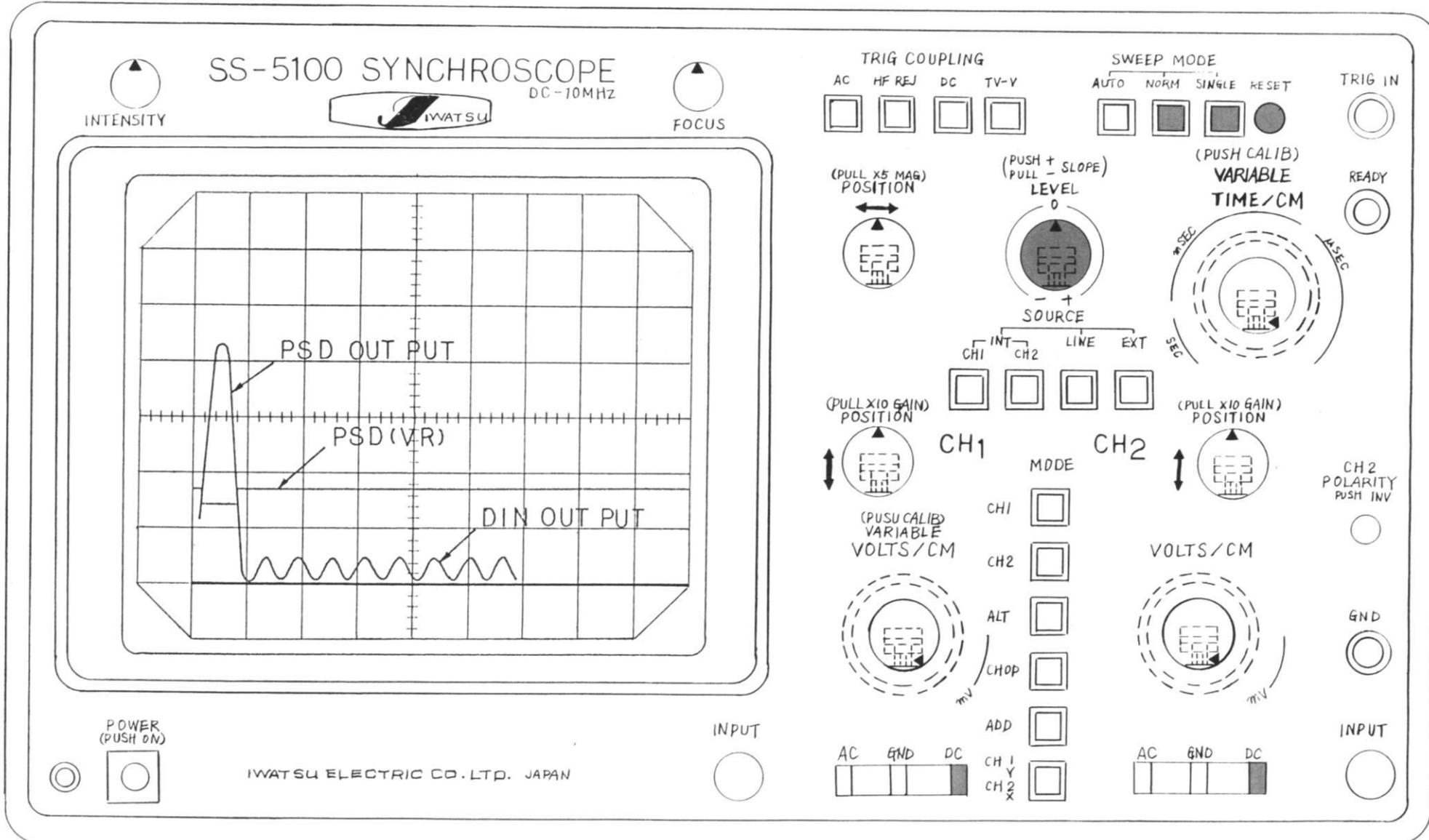
5. SETTINGS FOR CHECKING THE PSD TIMING
