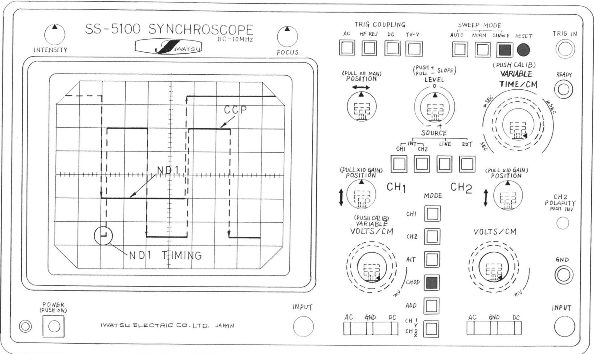
7 SETTINGS FOR CHECKING THE CPU BOARD
