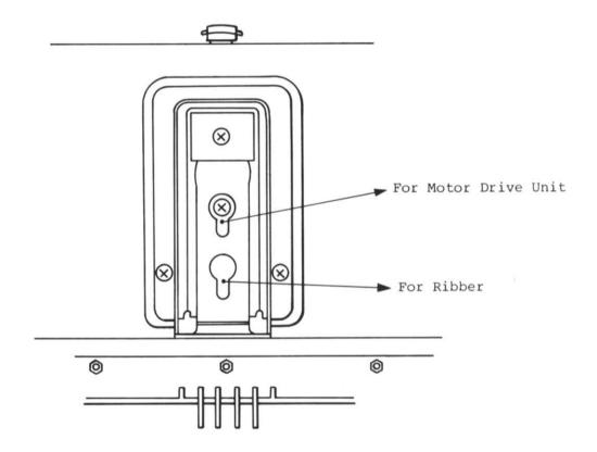
Note: When the Motor Drive Unit (SA-205) is used with the Model 150 knitter, the Yarn Rod muct be changed to the one exclusive to the Motor Drive Unit.
