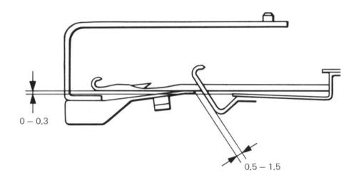
Y.S. (Measurement between the rear edge of the Yarn Feeder and the Sinker Post.) 0.5 - 1.5 mm (Adjusting method is same as for the Model 360 knitter.)
