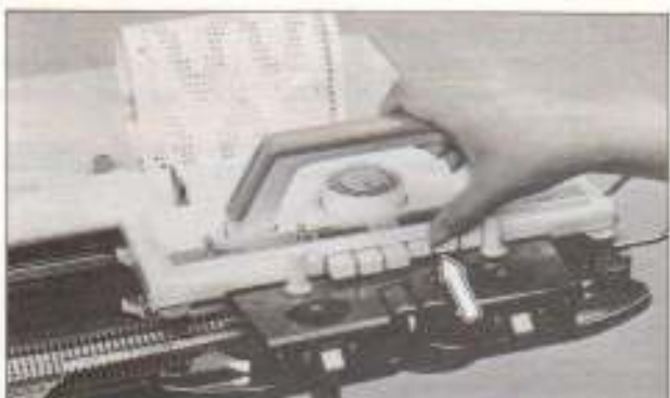
8. To select the needles, depress both "PART" buttons and set the CHANGE KNOB to K.C.
