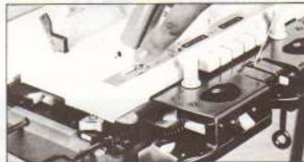
1. Set the HOLDING CAM LEVER of the K carriage to position H.
