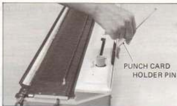
1. Insert the PUNCH CARD HOLDER PIN in the hole behind the slit.
