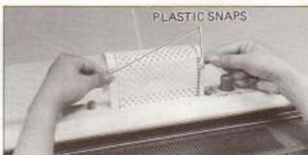
5. The card ends must be overlapped and clipped together with the PLASTIC SNAPS provided in the accessory box.
