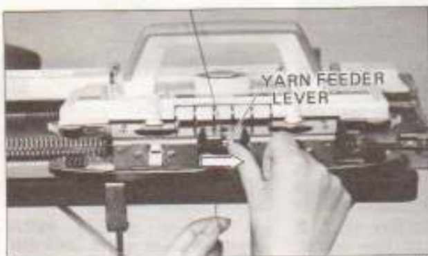
6. Hold the end of the yarn with your left hand under the YARN FEEDER "A". Close the YARN FEEDER LEVER.
