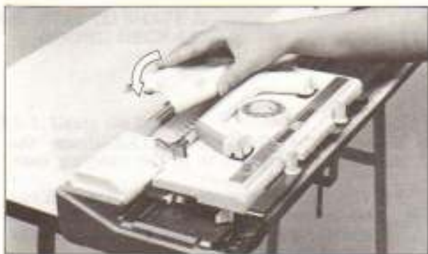
12. Replace the other accessories in the accessory box and close it. Push all needles back to position A.
