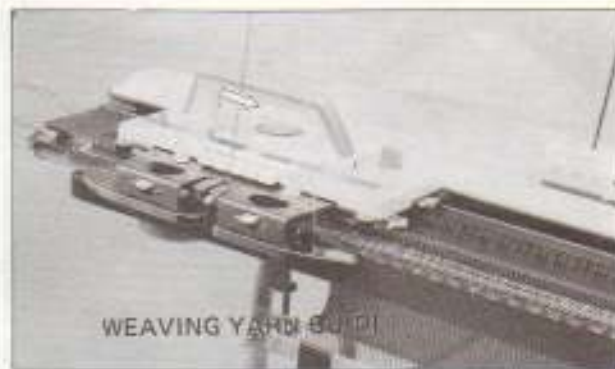
9. Move the K CARRIAGE to right making sure that the weaving yarn is in the right WEAVING YARN GUIDE.
