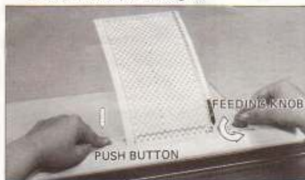
4. It is easier to turn the FEEDING KNOB by pressing down the PUSH BUTTON at the same time.
