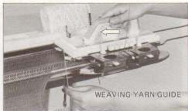
6. Make sure that the Weaving yarn is in the left WEAVING YARN GUIDE.
