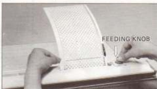
3. Make sure that the starting line is parallel to the panel. Press down the FEEDING KNOB and turn to left (to FEED) to feed the Punch card.
