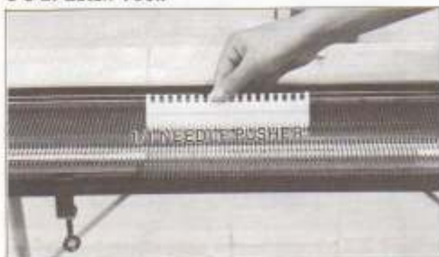
1. Place the K CARRIAGE to the right and bring forward to position E all the needles required.
