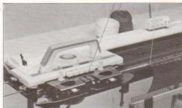
8. Transfer the Weaving yarn under the Carriage to the right WEAVING YARN GUIDE.
