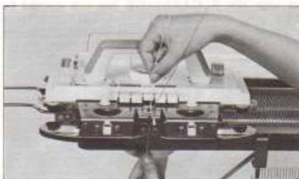
12. Thread the yarn into the YARN FEEDER and start the knitting again. When knitting, Fair-isle patterns or weaving patterns, do not forget to thread the second color yarn.
