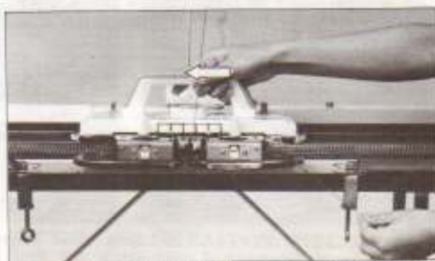
Move the K CARRIAGE to left holding the end of the yarn with your left hand. (When moving the K CARRIAGE, keep your left hand at the right edge of the Knitting).
