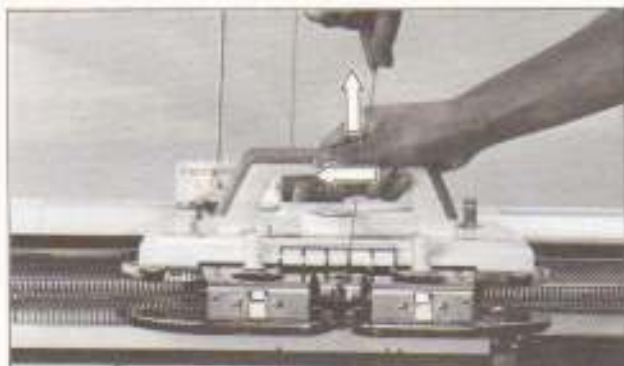
5. Move the K CARRIAGE from right to left lifting the yarn up slightly.
