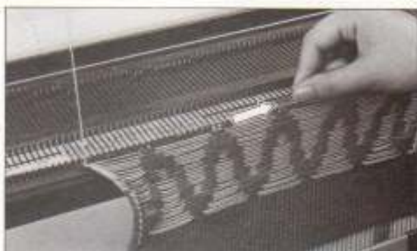
Unravel the main yarn the same way as the second color yarn.
