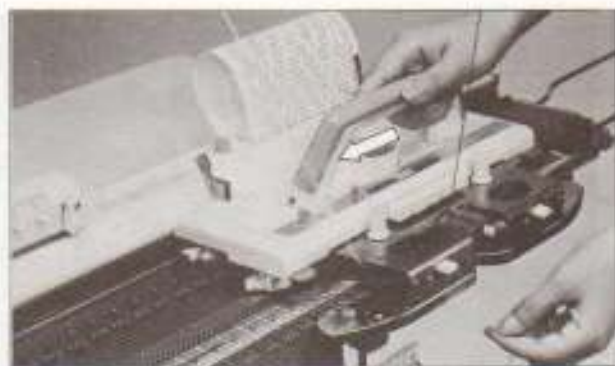
Hold the end of the Weaving yarn with your left hand. (Keep your left hand at the right edge of the knitting.) Operate the K CARRIAGE.
