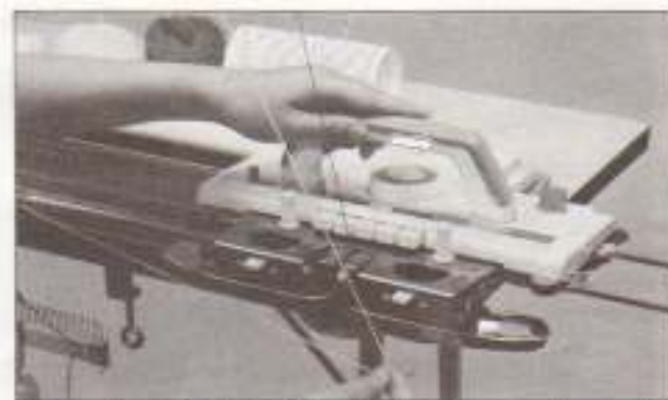
Move the K CARRIAGE slightly to the right and transfer the Weaving yarn under the Carriage and to the left WEAVING YARN GUIDE.
