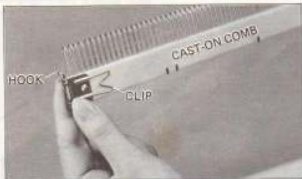
4. For casting-on, hang the CAST-ON COMB on the GATE PEGS of the machine.
