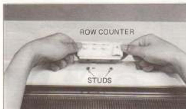
9. Setting up the ROW COUNTER on the two STUDS at the center of the machine. 1). Set the ROW COUNTER onto the two STUDS.
