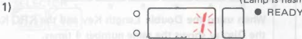
This indicates the needle selection for the first row has been done.
