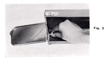
b. Fasten the automatic yarn feeder rod in the center screw hole at the rear of the knitter. Fasten the rod 4-5 threads, then fasten the lock nut while the stopper on the rod must be placed back side of the knitter. (See Fig.10 A, B)
