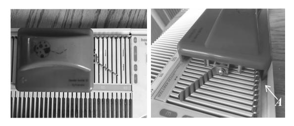
Leave the first 2 needles from the right in B position, push the next 2 needles to D position by hand, leave next 2 needles in B position, and then push 2 more needles to D position as shown.
