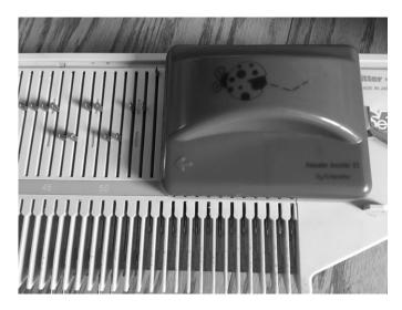
4. Slide the Needle Beetle across the needle bed towards the left. \*While sliding the Needle Beetle push the knitting against the machine by hand to hold it firmly in position. It will select the rest of the needles for you as it travels across the needle bed and pushes them into "E" position. \*Remember the Needle Beetle will only work when started from the right side and slid to the left side.
