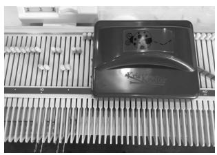
4. Slide the Needle Beetle across the needle bed towards the left. \*While sliding the Needle Beetle push the knitting against the machine by hand to hold it firmly in position. It will select the rest of the needles for you as it travels across the needle bed. \*Remember the Needle Beetle will only work when started from the right side and slid to the left side.
