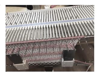
Set the Weave-R II on the needle bed as shown, on the carriage side, now push it across the needle bed. Don't push too fast as this could cause mis-patterning. A medium speed is fine.
