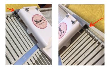
All the needles in B position and E position are now aligned into *forward D position*. You will see that your weaving yarn is now woven in between every other needle and held securely in place ready to be knit with main carriage.
