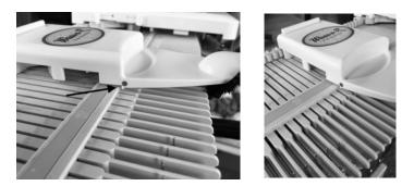
All the needles in B position and D position are now aligned into *forward C position*. You will see that your weaving yarn is now woven in between every other needle and held securely in place ready to be knit with main carriage.
