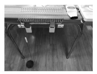
Set the Weave-R on the needle bed as shown, (Red dots are on the Weave-R to make placement against front rail quicker/easier to see) on the carriage side, now push it across the needle bed. Don't push too fast as this could cause mis-patterning. A medium speed is fine.
