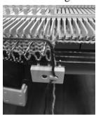
5. Manually Push or use needle selector tool to push every other needle to D position. OR
