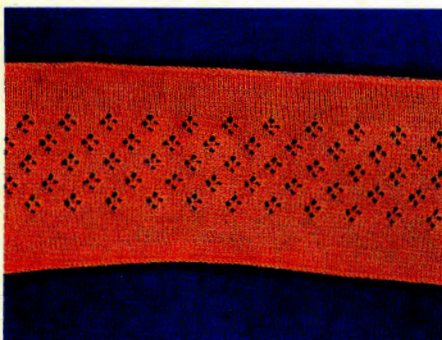
Lace stitches with a small number of L-Carr movements have a very similar structure to stocking stitch.
