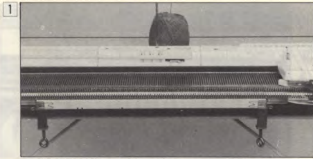
1 Hang the CAST-ON COMB onto the GATE PEGS.
