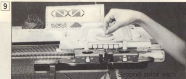
Then, thread the second color yarn which was clipped under the YARN CLIP into the YARN FEEDER "A" Close the YARN FEEDER LEVER.
