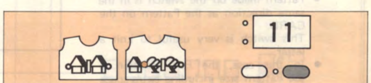
(K) Enter Green 11 which shows the left end of Pattern Width on swatch.
