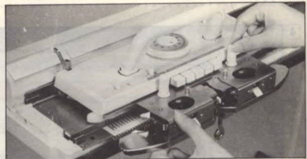
Press down the SPRING and remove the SINKER PLATE ASSEMBLY from the carrying case.
