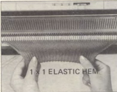
8 After knitting several rows, pull out the CAST-ON THREAD. The part knitted with the waste yarn is removed. The 1 x 1 ELASTIC HEM is finished.
