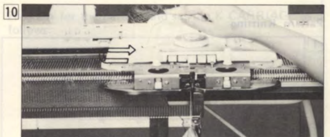
Knit two rows holding the end of the second color yarn under the YARN FEEDER with your left hand.
