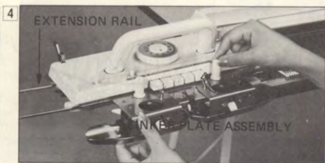
4 Place the K CARRIAGE on the EXTENSION RAIL and set the SINKER PLATE ASSEMBLY on the K carriage.
