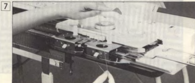
Change the yarn in the YARN FEEDER "A" with the second color yarn for two color patterns. K CARRIAGE is on the right side of the machine. Pull out the yarn in the YARN FEEDER "A". It is easier to remove the yarn by moving the K CARRIAGE to the right.
