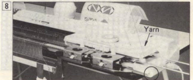
Hook the yarn taken from the YARN FEEDER "A" on the edge of the machine to hold it.
