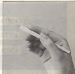
How to hold the latch tool.
