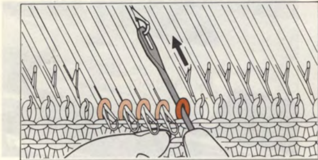
4). Push the TRANSFER TOOL toward the machine until the stitch is on the transfer tool.
