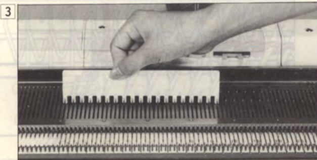
Using 1/1 NEEDLE PUSHER, bring forward every other needle to position D.
