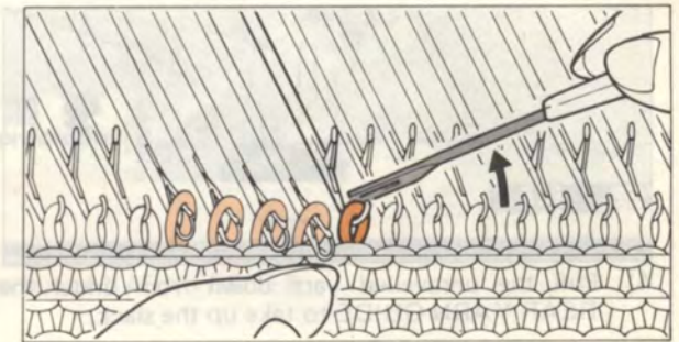
5). Transfer the stitch on the TRANSFER TOOL to the HOOK of the needle.
