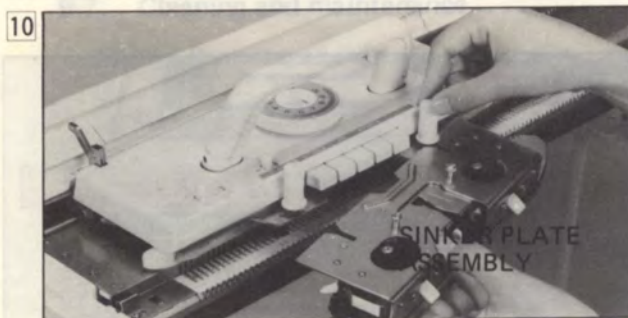
Set the SINKER PLATE ASSEMBLY up on the K CARRIAGE.
