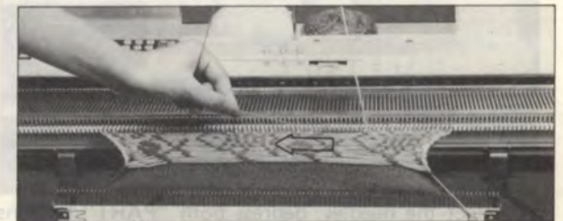
1). Hold the main yarn parallel with the GATE PEGS.
