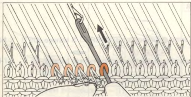
4). Push the TRANSFER TOOL toward the machine until the stitch is on the stem of the transfer tool.
