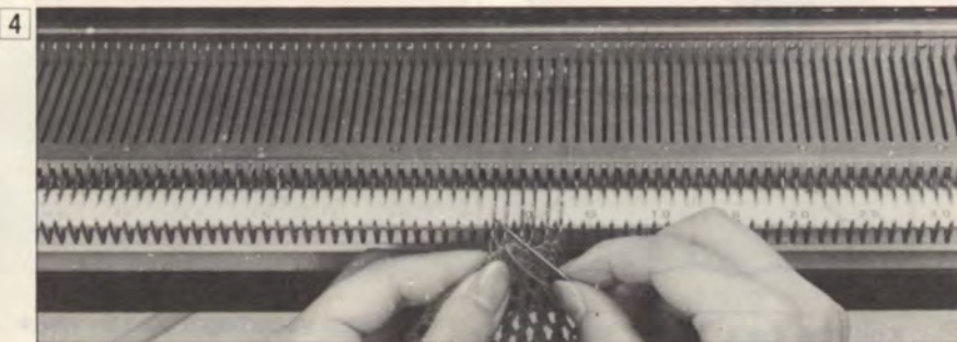
When parts (1) and (2) are completed, bring the needles for part (3) to position B and bind off.
