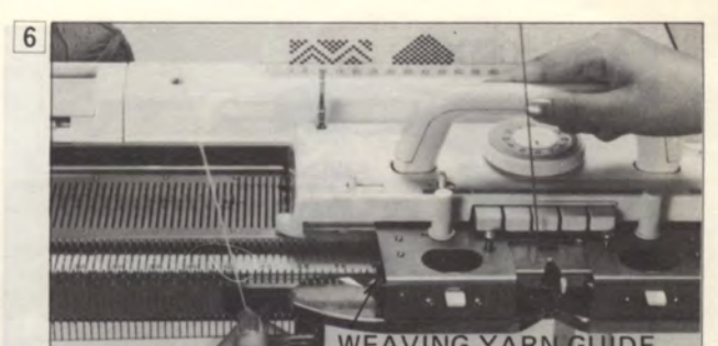
6 Make sure that the weaving yarn is in the left WEAVING YARN GUIDE.
