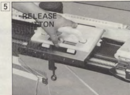
5 Remove the L CARRIAGE from the machine by pushing the RELEASE BUTTON.
