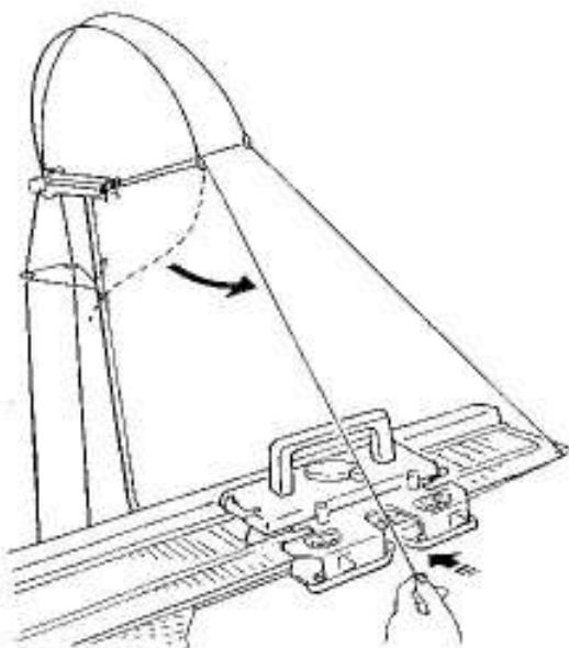
Remove the second colour yarn from the Yarn Clip and place it in the Main Yarn Feeder.
