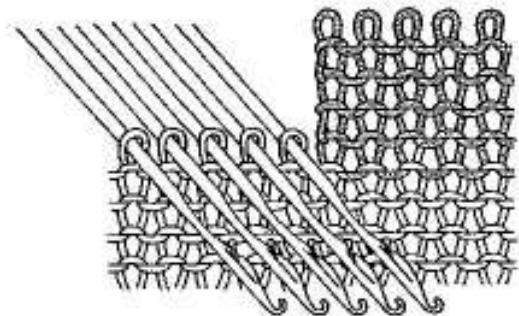
2. Thread waste yarn into the Yarn Feeder and knit several rows.
