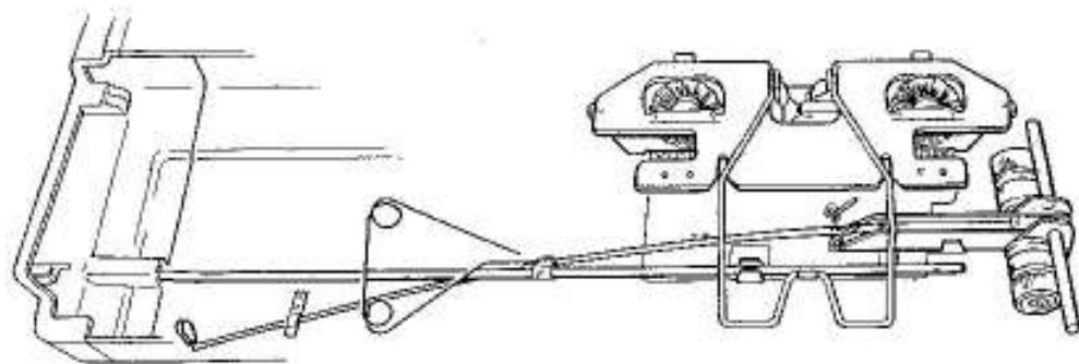
Remove the Auto Tension and Arm from the Knitter and pack them inside the Top Cover.
