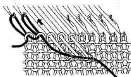
2. Starting with the end needle, push the needles back to A position manually.
