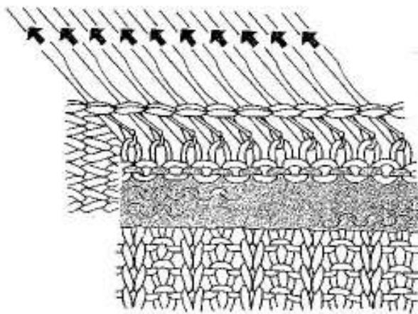
3. Push back the needles to B position, leaving one stitch in the needle hooks.
