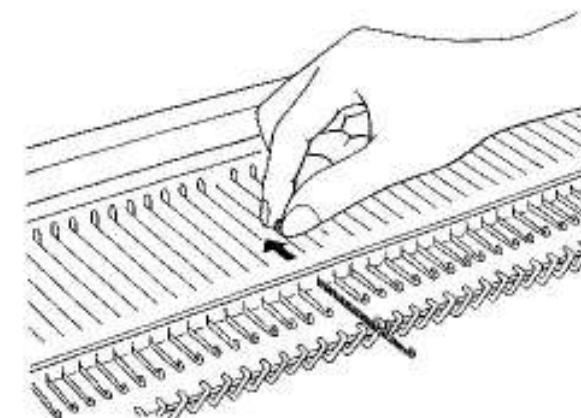
5. Push the needle back to A position by holding the butt.
