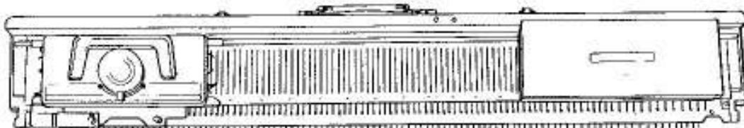
Place the Accessory Box on the right end of the Needle Bed.
