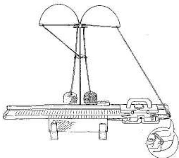
Place the main yarn in the yarn rest at the side of Needle Bed.
