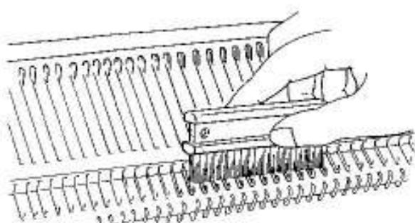
To clean your Knitter, remove the Carriage from the Needle Bed.
