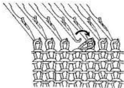
1. Place 1 stitch onto its adjacent needle. Leave the empty needle in B position.
