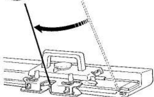
Remove the main yarn from the yarn rest and place it into the Main Yarn Feeder.
