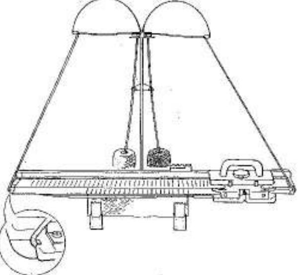
Remove the second colour yarn from Yarn Feeder and place it in the empty yarn rest.
