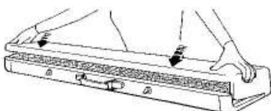
Place the Top Cover onto the Needle Bed.
