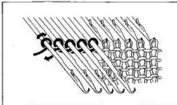
When the Carriage is at the left side, wind yarn around the needles in the clockwise direction.
