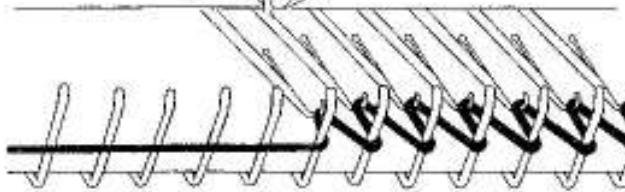
To correct, hold yarn above the Yarn Feeder and pull it down to allow some slack.
