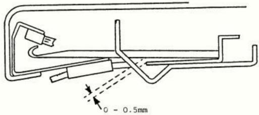
P.S. Measurement (Adjusted clearance between the slant face of the Sinker and the edge of the Fabric Pressers.)..... 1.3 - 1.8mm
