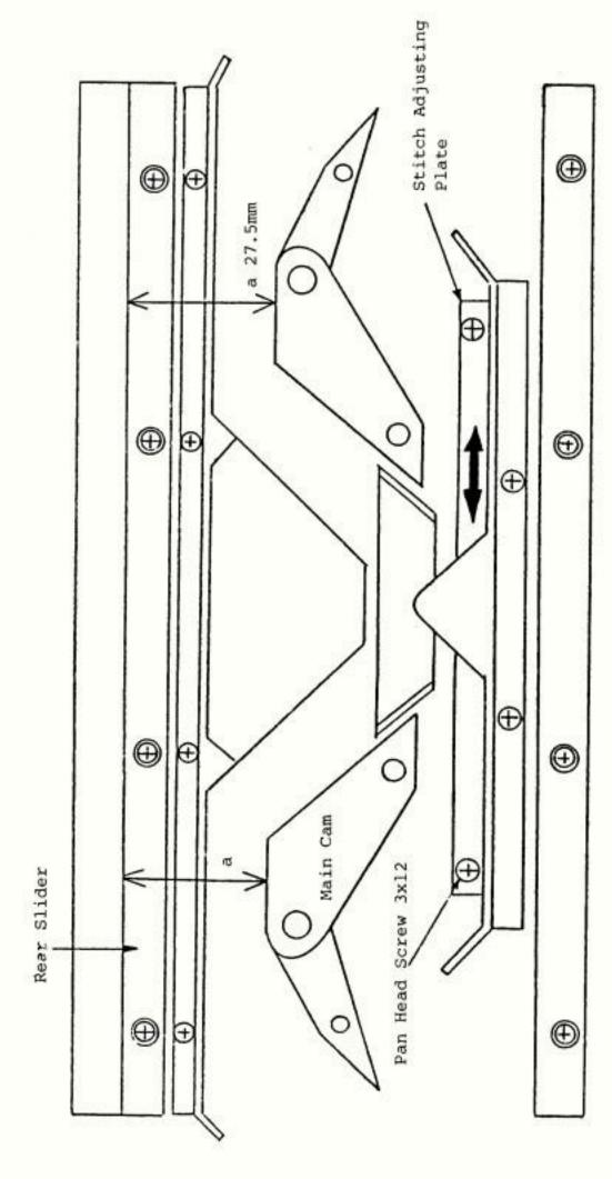
If the measurement for one main cam is different from that for the other main cam, loosen the pan head scerw (3x12) securing the Stitch Adjusting Plate, and move it to right or left to have the main cams into The position of the main cams is adjusted to 27.5mm from the rear slider when the Stitch Dial is set at 5. correct position.
