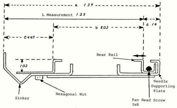
How to adjust the measurements of the needle bed
