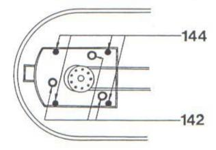
Insert the 4mm Allen key into one of the 3 screws (142) einstecken. 1.1.6 Push the motor by hand towards the profile bar and tight the screw (142). The tooth belt is now untightend.
