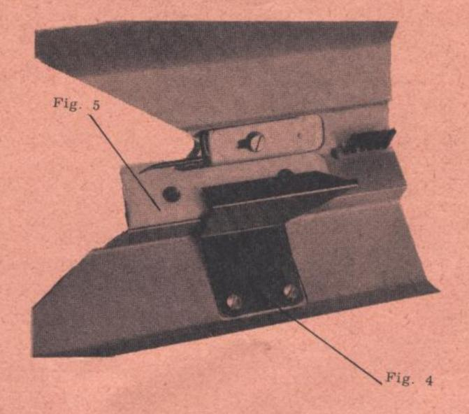
At first remove latch closing plate (Fig. 4) by unscrewing 2 screws. Then remove latch retainer (Fig. 5) by unscrewing 2 screws. Lay under or remove space plates respectively.
