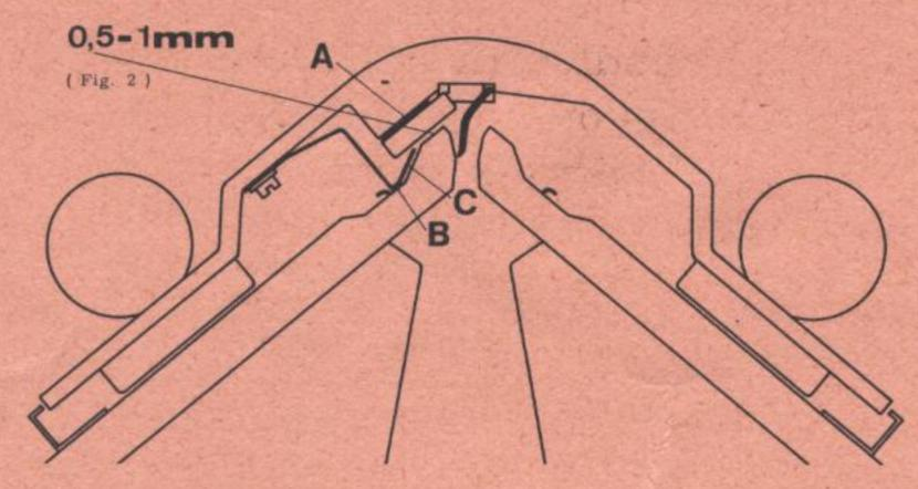
After adjusting tighten screws of latch closing plate completely.
