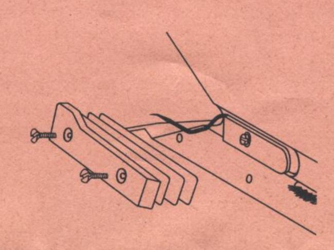
Fasten latch retainer and check distance on the machine. If o.k. temporary fasten latch closing plate.
