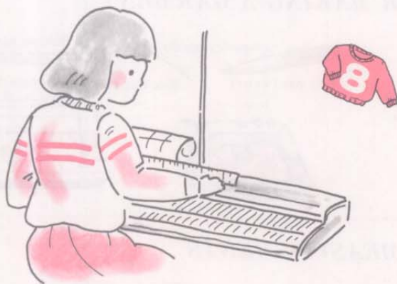
Set the Knit-leader according to the gauge.
