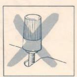
Ensure that the Arm Nuts fit properly into the cut-out of the Arm.
