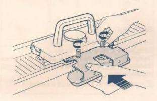
Remove the Arm from the packing and position it under the two Arm Nut screws.
