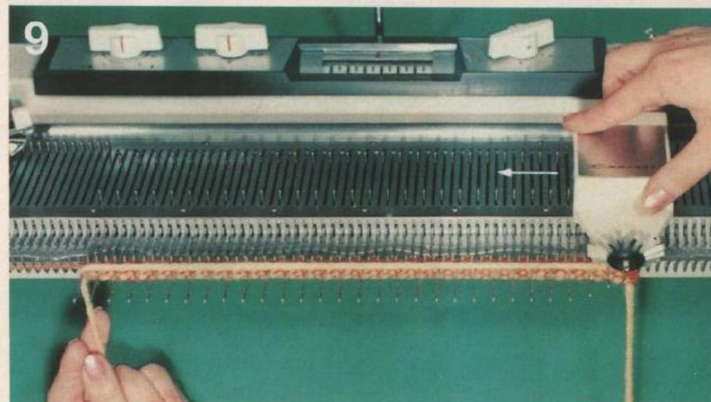
9 Lay the weaving yarn from right to left. Hold it slightly taut, and push the weaver from right to left. Repeat steps 5 – 9
