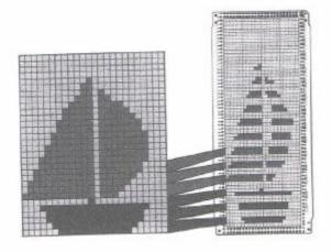
(2) Mark the parts of contrast yern on the first and second rows of the pattern onto the second and third rows of the Card (non-coloured rows) respectively.
