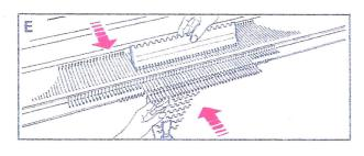
(4) Push all the knitting needles to holding position using the Needle Pusher. (Fig. E)
