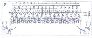
(5) Ease the fabric approx. 5mm away from the Sinker Posts and remove comb and/or weights if these have been used for the main knitting. (Fig. F)
