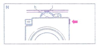
(7) By pushing in the red end of the Slide Button, the Connection Gear "h" will mesh into the Rack "i" of the needle bed, (Fig. H) if the Gear meshes with the Rack improperly, incorrect linking of stitches will be resulted.
