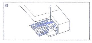
(6) Move the Linker to the right edge of the fabric till the SC Arm "g" comes behind the first 4 stitches. (Fig. G)
