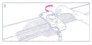
\* Is the Crank Knob being turned in the correct direction? (Fig. E)
