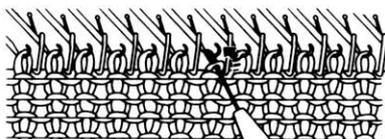
5. If stitches have slipped behind the latches of needles, use the Transfer Tool to replace these stitches in the needle hooks. Unravel the knitted stitches (see page 19) and align the needles in B position.
