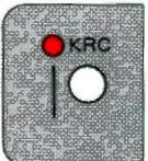
Push this key to knit in fairisle rib (jacquard) using the pattern data of fairisle. (Both the ribber and the double bed colour changer are necessary for fairisle rib.)
