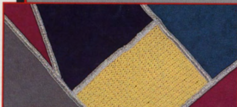
Flatlocked Seams allow mixing and matching of different fabric textures and colors using a decorative topstitch.
