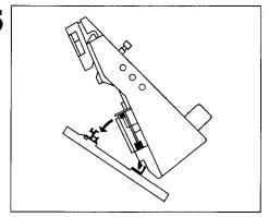
Place the casting off device TRI-COFIT onto the needle bed, to the right of the needles in Working Position, as follows:
