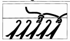
Push the locks without the feeding eyelet to the left end of the needle bed.
