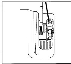
Insert the feeding eyelet into the TRICOFIT by first pulling the yarn between the feeding eyelet and the knitting from above to the back between the brush and the casing. Make sure the yarn lies underneath the decker needle.
