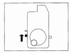
Move **the main lever up =** ""on". We recommend pulling the knitting down gently when doing this.
