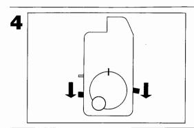
Handwheel knob with **both bars** in a line = "zero" position.
