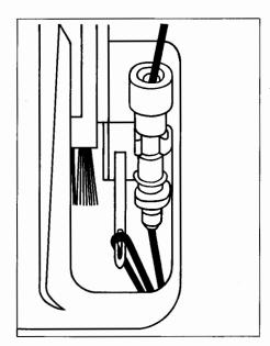
Set stitch counter to zero by turning each one of the three knobs.
