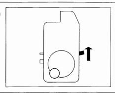
Before coming to the last three or four stitches, **push the stitch releaser up.** Continue to turn the handwheel until the TRICOFIT is past the actual knitting. Break off the yarn between the knitting and the TRICOFIT and pull it through the last stitch. Release the remaining stitches.
