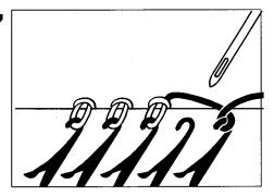
Move the TRICOFIT to the left until the decker needle points to the needle channel between the knitting and the needle round which the yarn was wound.
