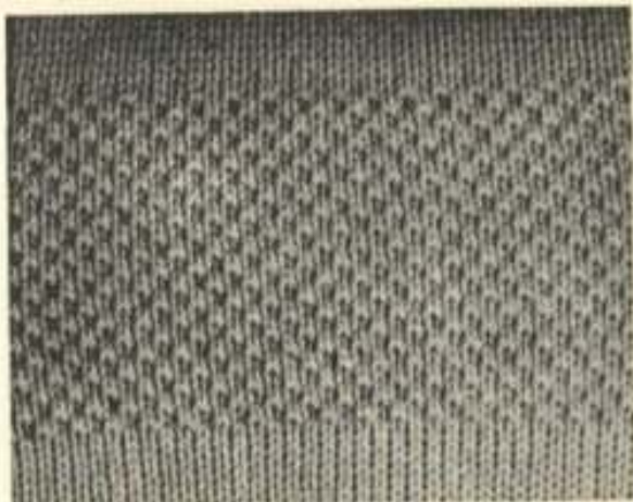
Tuck (in one direction) This pattern is reversible. Start with the carriage at the right side.
