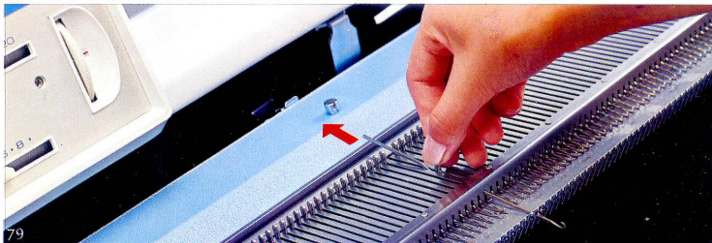
79 Pull the needle forward as far as it will go and down the hook of the needle until the shank of the needle is taken away from the needle bed, drawing it backwards and replace a spare needle. (See fig. 79)
