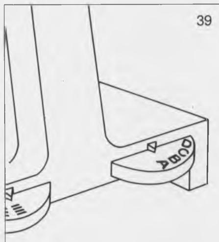
The back dial of the two dials on the right-hand side of the lock is called the **pattern selector**.
