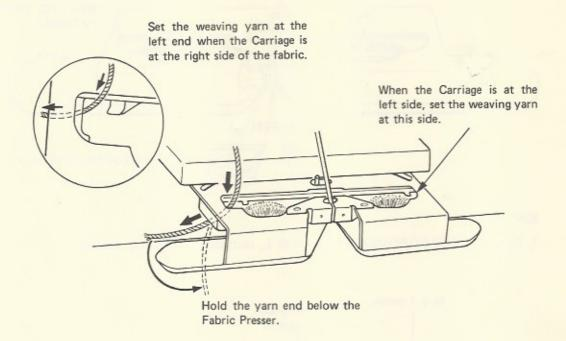
NOTE: When setting the weaving yarn into the Arm, place it at the side beyond the knitting yarn in order to avoid crossing of those two yarns.
