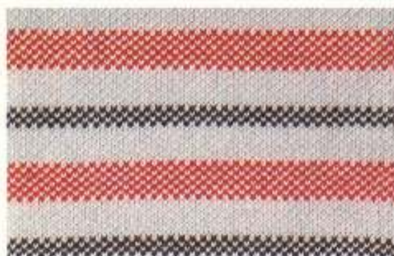
Card No. 1-A Col. 1-white Knit 8 rows col. 2-grey in feeder 2 Knit 4 rows col. 3-black in feeder 2 Knit 8 rows col. 2-grey in feeder 2 Knit 8 rows col. 4-red in feeder 2
