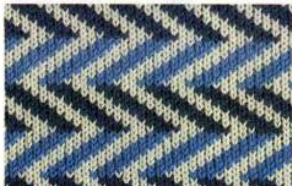
Card No. 18-A Col. 1-white Start knitting at 5 on card. Knit 8 rows col. 2-sky blue in feeder 2 Knit 8 rows col. 3-blue in feeder 2
