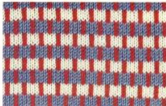
Card No. 13-A Col. 2-red in feeder 2. Knit 4 rows col. 1-white in feeder 1. Knit 4 rows col. 3-grey in feeder 1.
