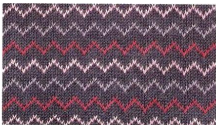
Card No. 3 After turning selector lever when no needle is selected, knit two rows of plain knitting and change to col. 2.
