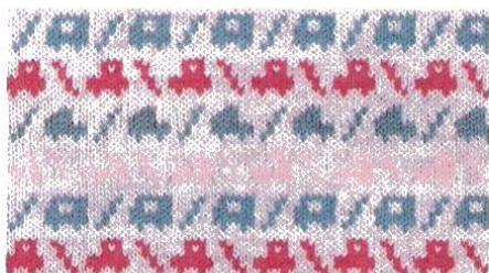
Card No. 6 After turning selector lever when no needle is selected, knit two rows of plain knitting.
