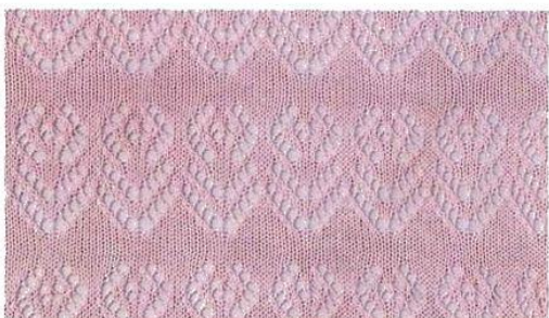
Card No. 19 10 \Leftarrow — Knit 10 rows of plain knitting. Turn selector lever and move lace carriage to Right.
