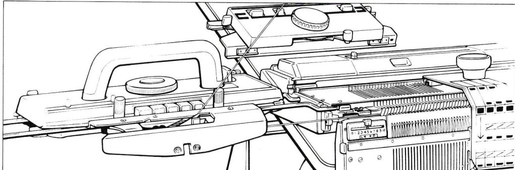
To avoid the mis-transferring the stitches, it is better to transfer the both end stitches by using the double eyelet transfer needle.
