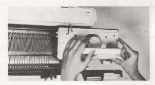
5 Pull forward carriage-release lever of main carriage. At rib carriage side, set main carriage on to the bed from front rail and then back rail. Set coupling.
