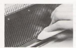
With a cloth or rag clean the rear rail of the needle bed, the front rail and the needle bed.
