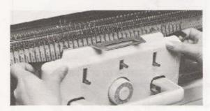
3 Pull both front holders of rib carriage.
