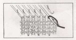
8 The needle latch must be open.
