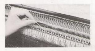
4 If there is any dropped stitch, see p. 45 Using transfer tool, set all stitches down to B position.
