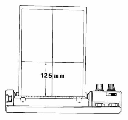
( I ). How to adjust in case 125 mm long Pattern Paper feeding accompanies less than 108 times Carriage operation.
